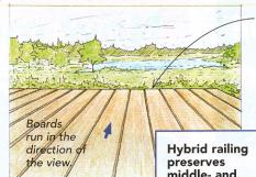
A railing is not required on a deck that's within 30 in. of the ground. Boards cantilever over supports, so there's no border.
