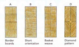
the decking joints and breaks the deck into sections. Simply orienting the decking in the shorter direction (B) de-emphasizes the length of the deck in an understated way. If you want the deck to be the center of attention, designs such as a basket weave (C) or diamond pattern (D) provide visual interest and draw attention away from the long, narrow aspect of the deck.
